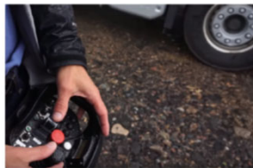
Figure 2.: Volvo external steering [22]
